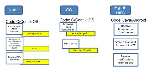
Figure 2: 6LowPAN Platform - key functionalities per functional component
